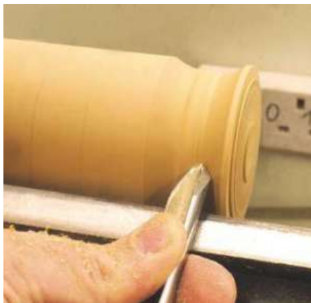
▲ Pic.8 Use the 13mm spindle gouge to define the top shape of the bowl. Put minimal shape on the outside at this stage, so as to maintain the strength for interior hollowing
